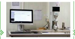
Universal Testing Machine: To test the mechanical property of MDF and other wood based panel products.
